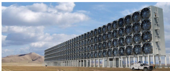
Figure 11 - DAC units assembled as larger unit (concept)
