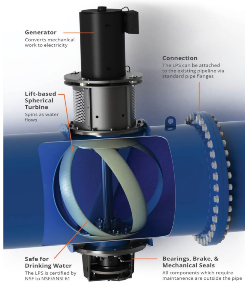
Figure 15 - Hydrodynamic Turbine (Lucid Energy)
