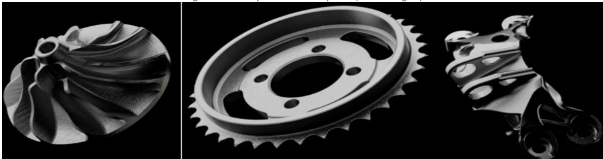
Figure 20 - Metal parts made from Selective Laser Melting
