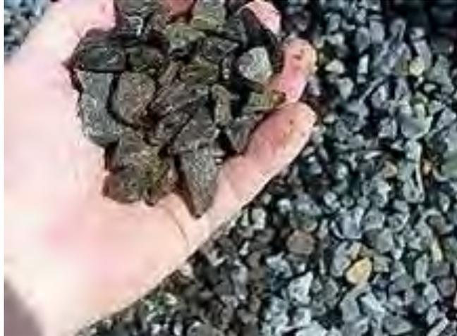
Figure 1. EAF steel slag aggregate. (from [en.wikipedia.org/wiki/Construction](http://en.wikipedia.org/wiki/Construction))
